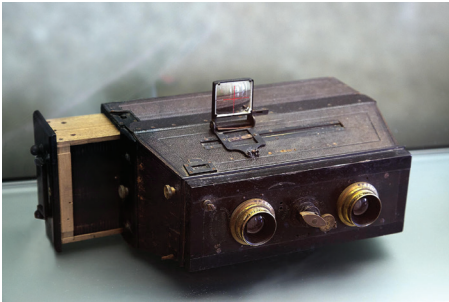
Fig. 30 The stereoscopic camera of Aurélio da Paz dos Reis. Mackenstein, Paris, France, circa 1906. Displayed at the Portuguese Centre of Photography, Porto. Carl Zeiss lenses f: 1.8/110 mm, single-speed and focal plane shutter; collapsible sports viewfinder; wooden chassis encased in leather. Photographic print created by Renato Roque.
