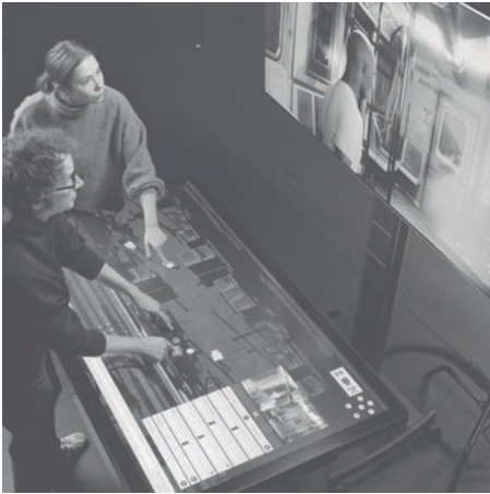
Image 1 – The cineDESK touchscreen displays the top view of a virtual location and the separate monitor shows the output of the active virtual camera (© Marco Quandt ZHDK 2022)
