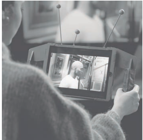
Image 4 – A position tracked tablet can be used as a hand-held camera controlling the virtual camera on the cineDESK (© Marco Quandt ZHDK 2022)
